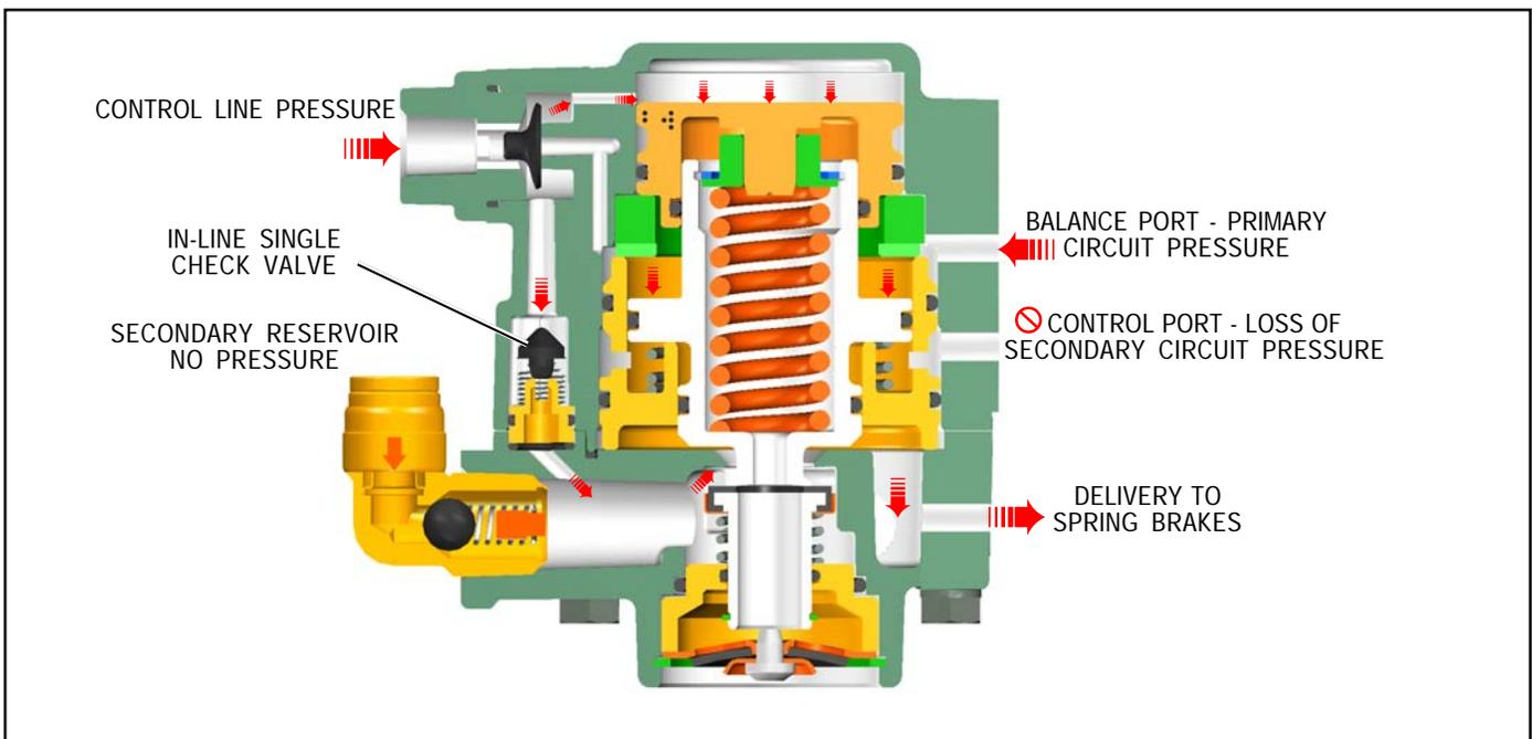
FIGURE 10 - SERVICE APPLICATION LOSS OF SECONDARY CIRCUIT
