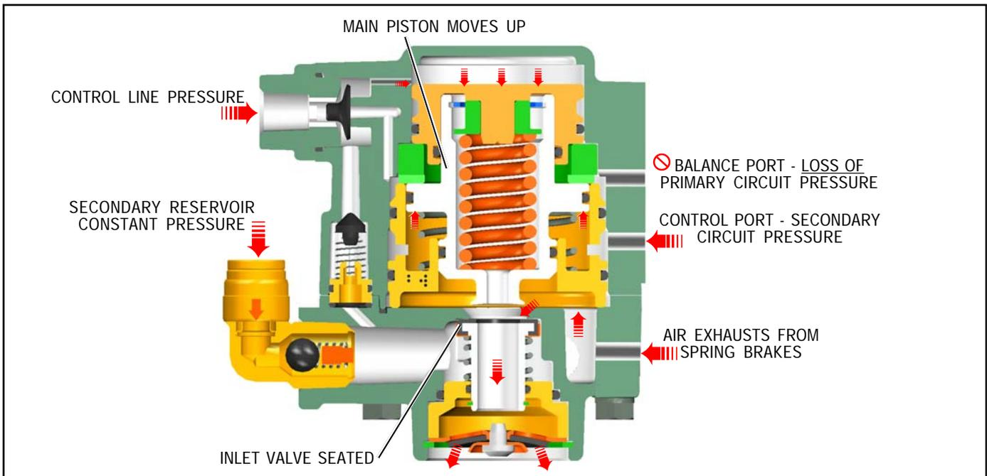
FIGURE 9 - SERVICE APPLICATION LOSS OF PRIMARY CIRCUIT
