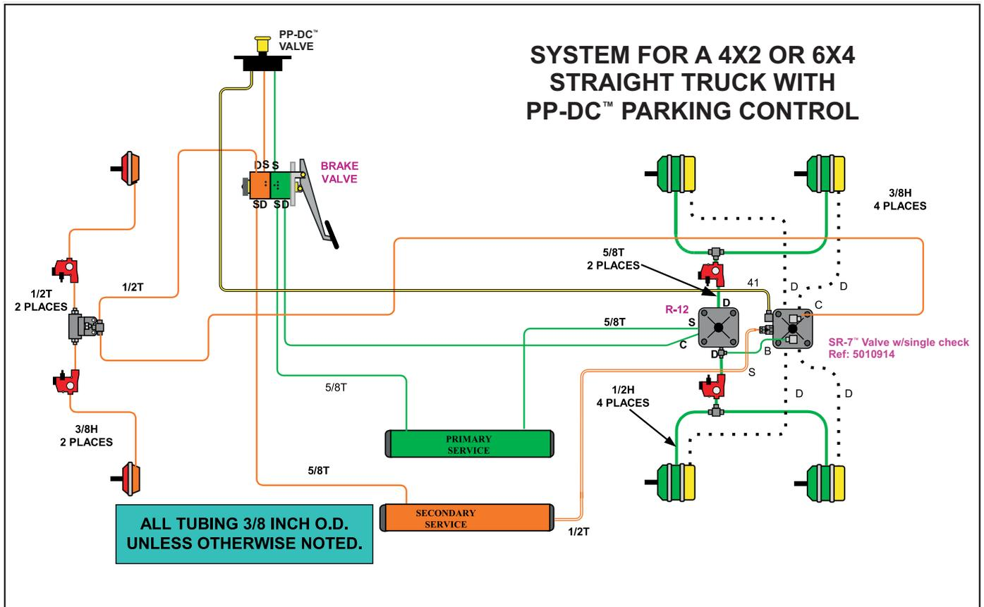
FIGURE 3 - SYSTEM SCHEMATIC WITH PP-DC™ PARK CONTROL
