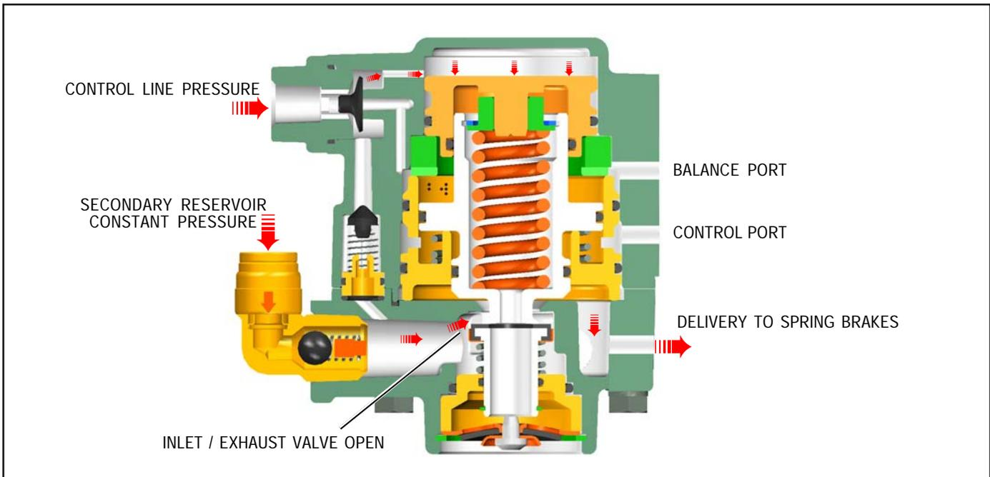
FIGURE 5 - CHARGING LESS THAN 107 PSI
